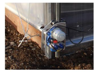
(Reversing the motor wires within a junction box, at the controller or at the drill battery terminals, will change rotational direction.)
